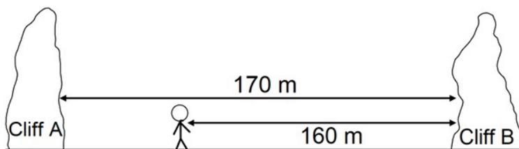
In the above diagram Lata stands between two cliffs and claps her hands. Determine the time taken by her to hear the **first** echo. Speed of sound in air  $320 \text{ ms}^{-1}$ .
