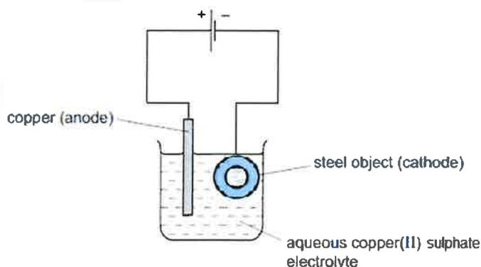
1. The chemical process taking place on the surface of the object is  $\text{Cu}^{2+}(\text{aq}) + 2\text{e}^- \rightarrow \text{Cu}(\text{s})$
